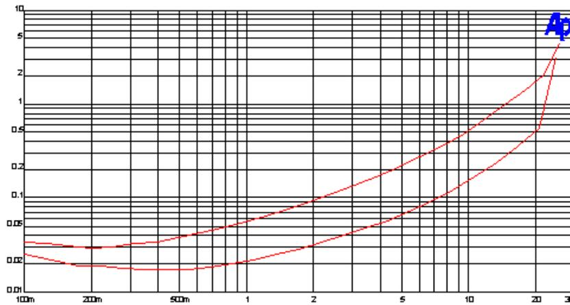
Harmonic distortion vs power at 500 Hz, 8 ohms, w/ and w/o feedback
