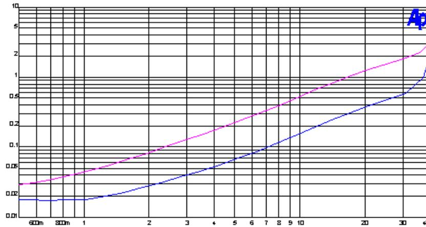
Harmonic distortion vs power at 500 Hz, 4 ohms, w/ and w/o feedback
