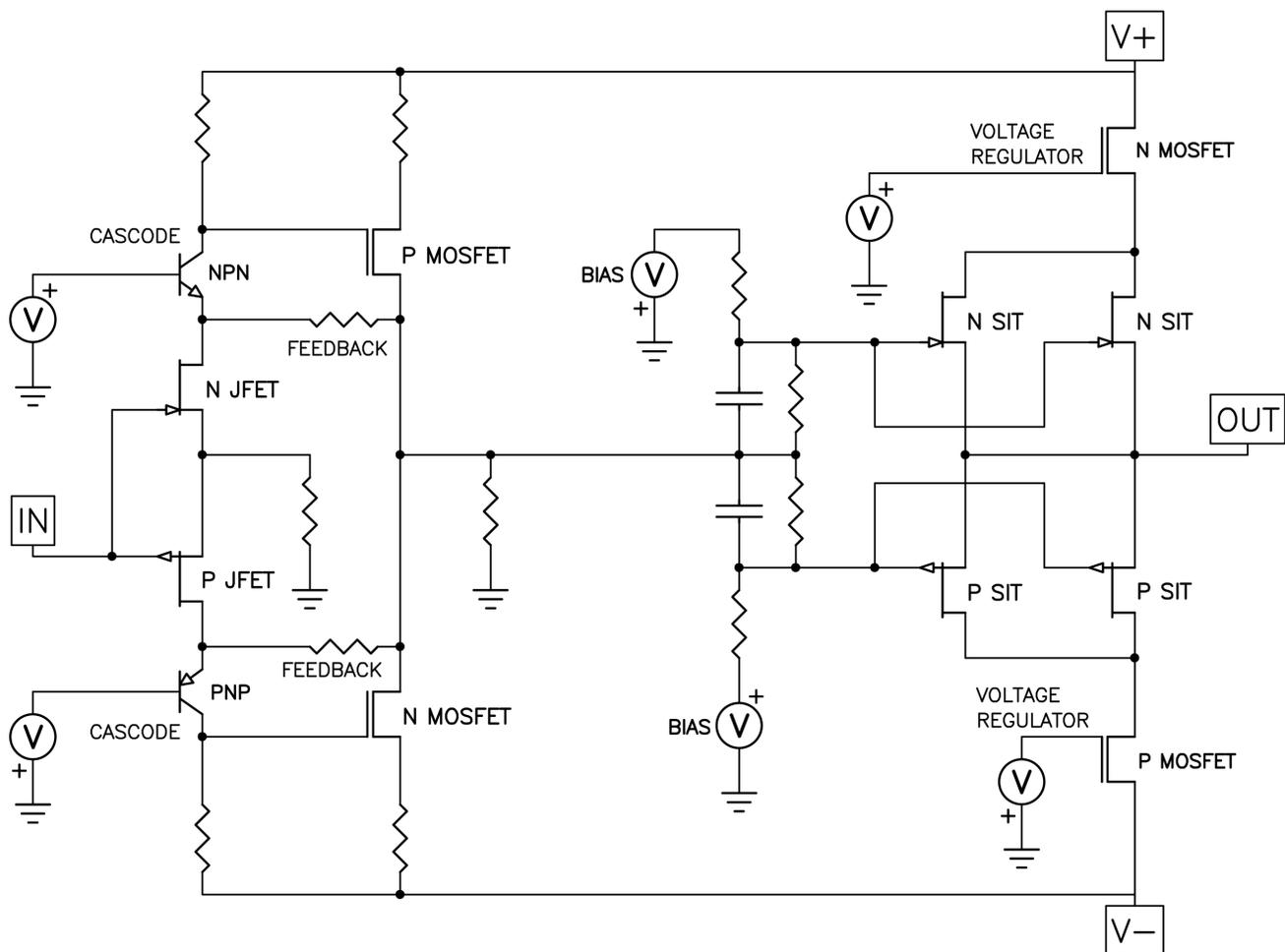
On the left side, the voltage gain stage, we can see new elements. We have *degenerating* resistors in series with the Source pins of the MOSFETs to lower the gain and stabilize the bias current against temperature drift. We have also introduced *Cascode* transistors for the input JFET devices and biased them with some constant voltage sources, and we have also introduced local *Cascode feedback* to linearize the gain and lower the output impedance of the front end.
