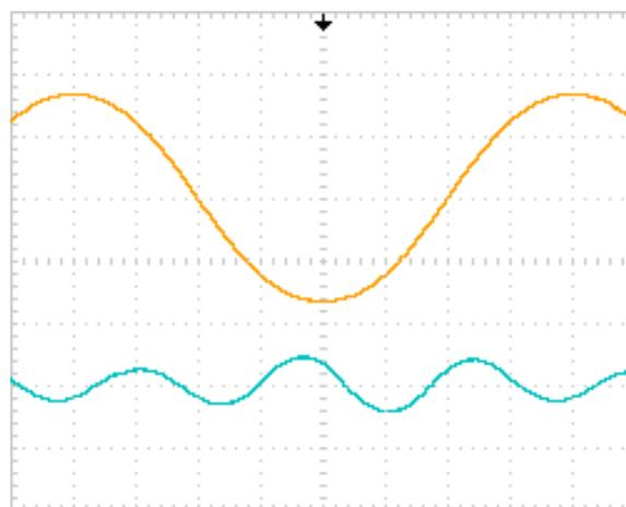
2% harmonic distortion waveform at 35 watts, 500 Hz, 4 ohms, w/o feedback
