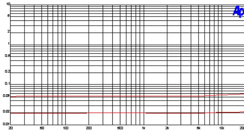
Harmonic distortion vs frequency at 1 watt, 8 ohms, w/ and w/o feedback
