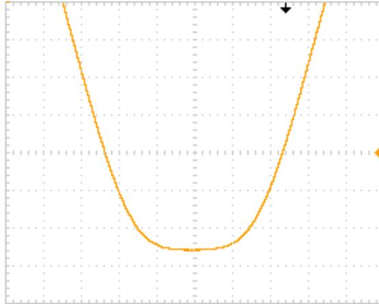
Current through positive output stage while the negative output stage delivers 3 Amps peak (40 watts peak @ 4 ohms). The minimum current is 0.1 Amps
