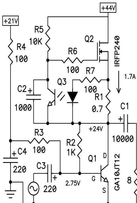
You can see a constant current source provided by Q2, R1, R5, R6, R7, C2 and an opto-isolator Q3 used as a current regulator. This circuit provides a relatively constant amount of DC current to bias Q1, the transistor of interest. Current through R1 develops about 1.1 volts across the LED portion of the opto-isolator which emits light that turns on the photo sensitive transistor of Q3 and this forms a feedback loop around Q2 which regulates the current.
