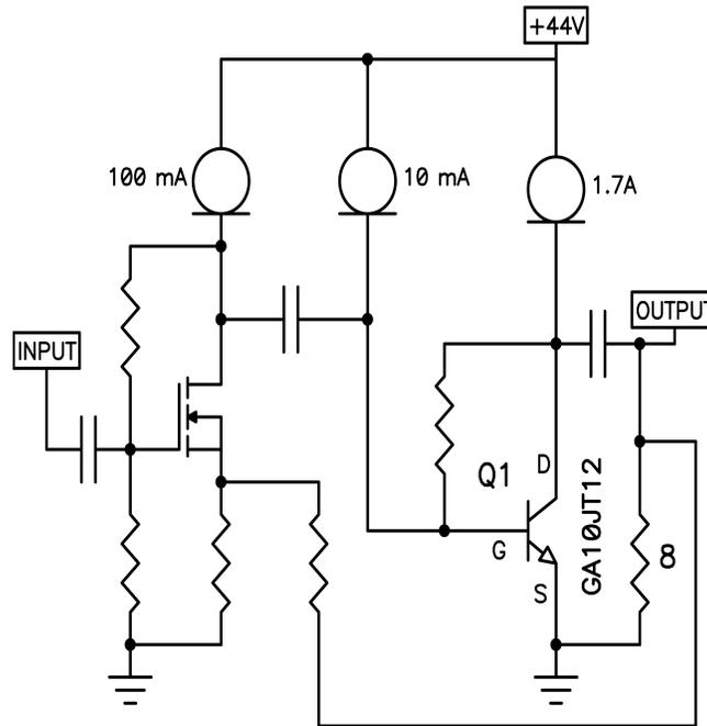
This should not be considered the best possible circuit, but is intended to illustrate an approach where a current source input and feedback to the GA10JT12 might be simply achieved. Alternatively, you can control the bias and feedback with an op-amp circuit.
