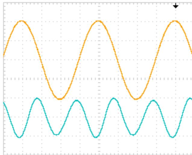
DISTORTION WAVEFORM AT 1 WATT
