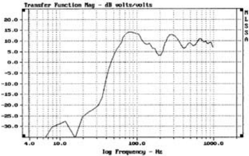
FIG 6 Near Field Bass Response in Horn
