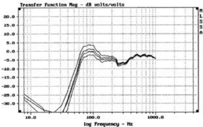
FIG 8 Listening Position Bass With High Pass Filters
