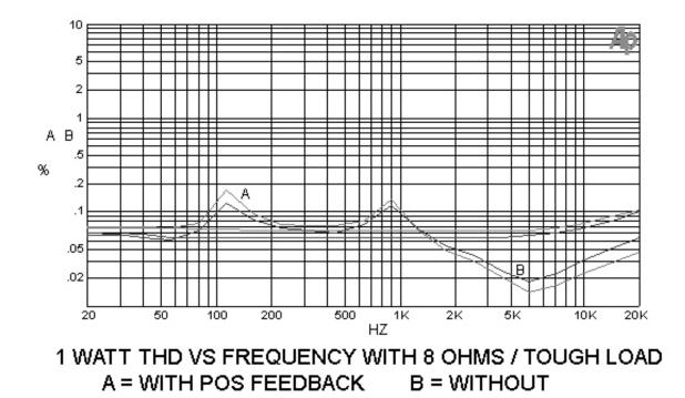
It is understood that pcf allows for slightly more distortion in proportion to the amount of positive feedback employed. Another way of viewing it is that the amount of positive feedback is subtracted from the negative feedback, and so the result is similar to simply having less negative feedback in the first place, in this case the amount being about 2 dB, which is not much at all.
