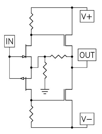
In such a simple circuit, there are opportunities for improving performance by careful choice of transistors, resistor values, voltage and current values and precise matching of parts. I built up a number of such amplifiers evaluating both the measurements and the sound, and after a while a very nice little amplifier emerged. That it (and the F5) resembled Plantefeve's *Profet* was testament to his fine work.
