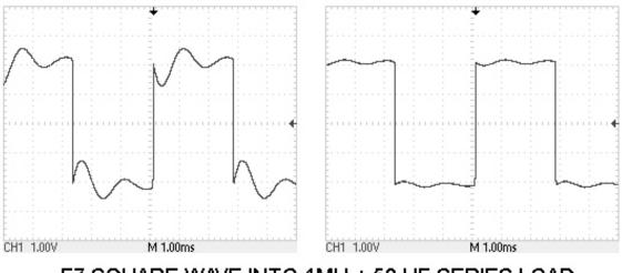
F7 SQUARE WAVE INTO 1MH + 50 UF SERIES LOAD RIGHT = WITH POSITIVE CURRENT FEEDBACK I also created a difficult test load reflecting an amalgam of the sorts of things seen in several popular loudspeakers. Here is the impedance of that load, dipping down below 3 ohms at two points:
