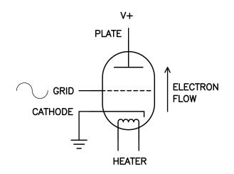
Triode operation is simple. Electrons have what's known as "negative electrostatic charge", and it is understood that "like" charges physically repel each other while opposite charges attract. The Plate is positively charged relative to the Cathode by a battery or other voltage source, and the electrons in the Cathode are attracted to the Plate, but are prevented by a natural tendency to hang out inside the Cathode and avoid the vacuum.
