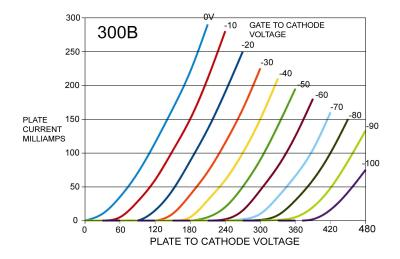
These curves show that the current from Cathode to Plate is a function not only of the Grid to Cathode voltage, but also of the Plate to Cathode. More positive Grid voltage and/or Plate voltage means more current flow. This dependence on the Plate voltage is often referred to as the "Plate impedance"
