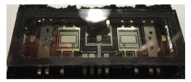
It's small, about 1 by 2 inches, and operates at power consumption of about 20 milli-Watts (including heater!). You can adjust the Grid bias point so as to create the effects I have described, and in my example Nutube circuit there is a potentiometer just for that. Here is the curve with the negative 2<sup>nd</sup> harmonic set at 1.7% at 1 volt out:
