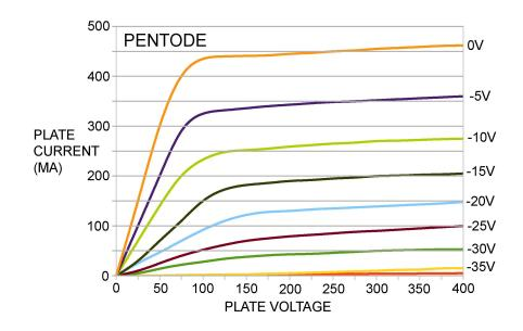
The extra control pins are used to flatten out the curves as you can see here, resulting in a higher Plate impedance for the tube, that is to say less current variation with Plate voltage. There's a specific performance advantage to this in many applications, but not in this discussion.
