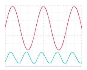
Compared to the fundamental, there are twice as many peaks and dips in the 2<sup>nd</sup> harmonic – it is at twice the frequency.
