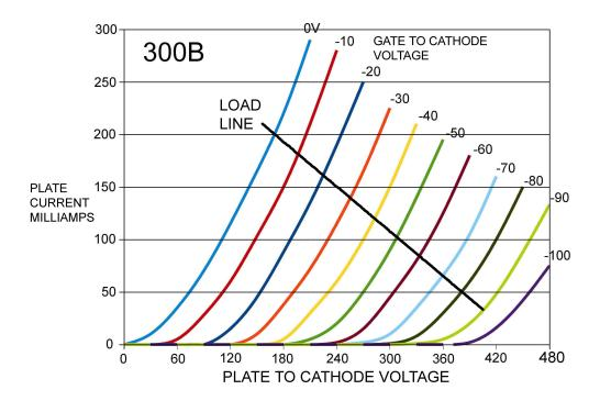
In this graph, we see the load-line for 300B Triode driving about 1800 ohms. This output could be passed through an output transformer which converts it into about 4 watts into an 8 ohm loudspeaker. When the Triode amplifies musical signal, it moves around on this line – if the load is a resistor. If if it is driving a speaker, or other reactive load like a capacitor or inductor, the varying impedance will make it wander around a bit.
