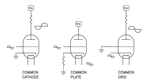
In Common-Cathode mode the tube amplifies both voltage and current in response to a signal voltage on the Grid. The output appears amplified out of phase into a load at the Plate. In Common-Plate mode the Cathode output voltage follows the Grid voltage, increasing the current only, in phase without voltage gain. In Common-Grid mode the input signal current is fed into the Cathode, and the output appears on the Plate, voltage amplified in phase, but with the same amount of current as the input.
