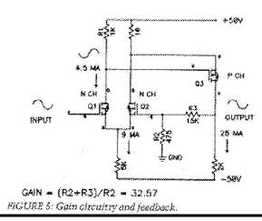
pull down the output of Q3, which by itself can supply only positive voltage and current, and it allows for negative output, providing "bias" for Q3 and placing it in a useful operating region.
