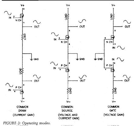
The third way to use a MOSFET is with common-gate operation, which has voltage gain but no current gain. Input appears at the source; output appears at the drain. This connection is most popularly used to form cascode operation, in which a common-gate device shields a common-source device.
