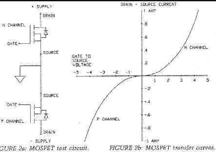
response to positive gate voltage, with respect to the source voltage (fig. 2b) If you wish more current, make the gate-to- source voltage more positive (for less, make it less positive). Conduction in the N-channel MOSFET will start generally at about 4V: less than 4V, no current; more than 4V, current flows.
