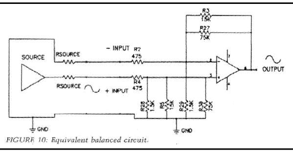
At the positive input, this is also the impedance seen by the signal, since the positive-input network is not attached to the amplifier output, and the impedance is passive. At the negative input, however, both the network's passive impedance and what is happening at the output form the input impedance.
