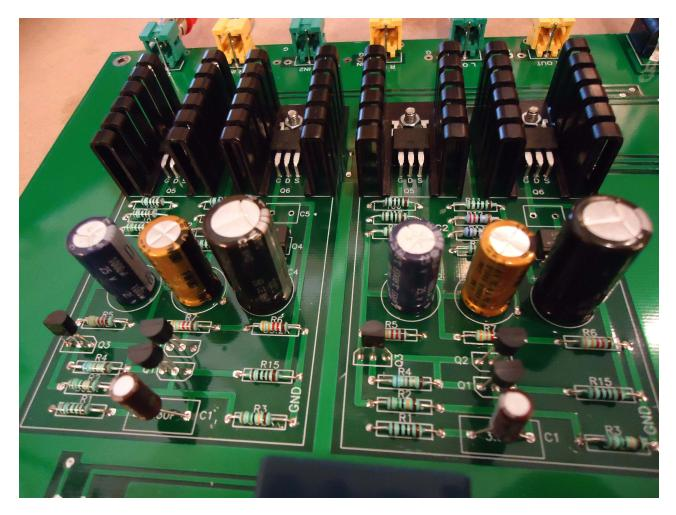
Notice also the orientation of the transistors, and remember the dot on the opto-isolator.
