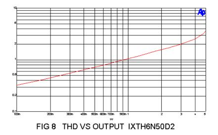
Definitely better, no? We pause in rejoicing to note that the IXTH6N50D2 has a little more input capacitance which is also more non-linear than the IXTH20N50. This will raise the distortion at the top end if driven by a preamp with a high source impedance, otherwise the distortion figure should be flat across the audio band.
