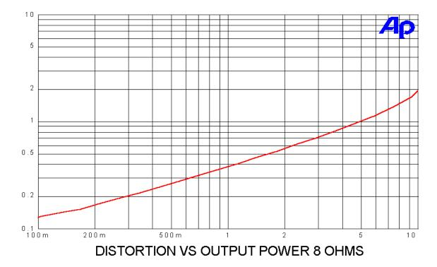
Here is a graph of that distortion vs output watts into 8 ohms:
