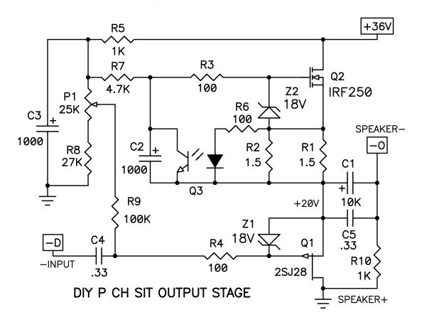
Q1 is the VFET gain device, Q2 is an N channel power Mosfet used for the constant current source, and Q3 is an opto-isolator wired to regulate the current through Q2. The Zener diodes are there to protect the Gate pins of Q1 and Q2 from high Gate-Source voltages which could damage them.
