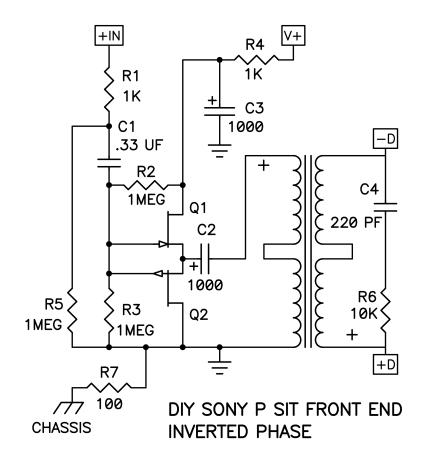
This circuit is mounted on a separate board from the output stage, and consists of a pair of complementary Jfet followers which drive the primary coil of the Edcor 600/15K step-up transformer. The Jfets are selected Toshiba 2SJ108 and 2SK370, the same chips as 2SJ74 and 2SK170 but in a smaller package, which provides for an input impedance to the amplifier of 330 Kohm and low distortion.
