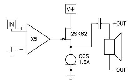
You will want to note that in addition to alterations of part locations, the signal phase has been changed. The X5 front end no longer inverts the signal and the phase of the loudspeaker connection is also now non-inverted. This is because the 2SK82 gives us the desired polarity of the 2<sup>nd</sup> harmonic distortion we want without needing the double inversion of the Part 1 2SJ28 VFET circuit.
