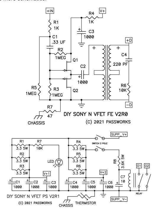
You will note the more elaborate filtering, made necessary by the VFET's exposure to rail noise and the larger thump of the circuit on turn-on/off.
