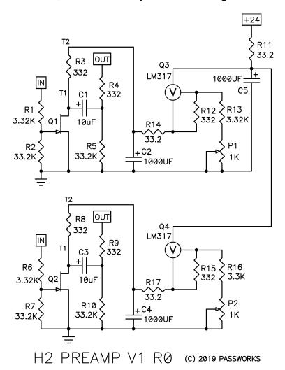
The J112 Jfet has been chosen as a suitably cheap choice and carefully matched out of a population with a 2.5V to 3.0V pinch-off voltage and an Idss of 30+ mA. In this circuit this Jfet itself has a voltage gain of about 14 dB, and could easily serve as a preamp with a volume control and such. You can use R1 and R2 as an input voltage divider, and if you replace R1 with 33.2K and R2 with 7.5k you will have unity gain.
