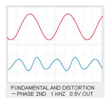
The red fundamental goes up and down at a 1 KHz rate, and we see that the blue wave goes up and down as well at twice the frequency, but aligned with the red wave in a particular way - the blue goes negative on all peaks of the fundamental. This as *negative phase 2<sup>nd</sup> harmonic*.
