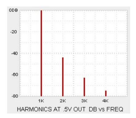
Above is what the spectrum looks like at 0.5V output, where you can see the relative amounts of 2<sup>nd</sup>, 3<sup>rd</sup> and 4<sup>th</sup> harmonics. We note that the 3<sup>rd</sup> is down about 18 dB from the 2<sup>nd</sup>, and the 4<sup>th</sup> is lower yet. This is approximate, and varies a bit between Jfet parts. This is very dependent on the voltage at T2, and can be adjusted over a fairly wide range.
