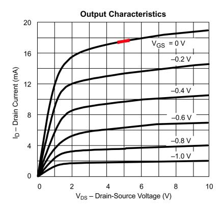
All these values depend on the others, and the angles, distances and curvature of the plotted lines tells us things about how the transistor behaves. The distance between the plots tell us the gain of the device at that spot, the angles of the lines tells us how the Vds affects the gain, and the curvature and uneven spacing of the lines show us the non-linear distortion of the device in any given area.
