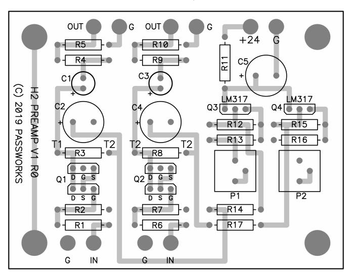
You will note that on the board are test points labeled T1 and T2. If we want to set up the H2 without a distortion analyzer, then you will be adjusting the voltage values at T2 while adjusting P1 and P2.
