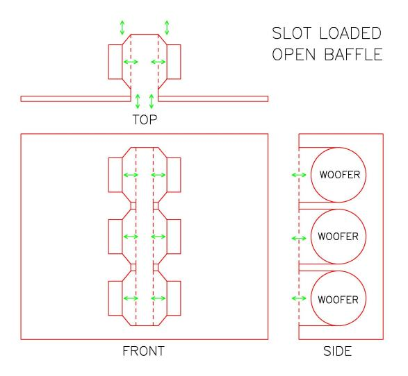
As an aid to understanding, I have highlighted the direction of air motion in this system with green arrows. The woofers are wire in phase and move toward and away from each other squeezing the air between them, and the pressure makes the air flow fast out the front. The air in back is not squeezed, and so flows more slowly out the rear.
