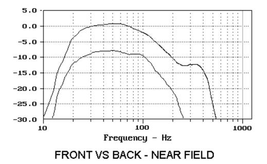
Unfortunately, this is only the difference you will experience in the close near field. As you move away from the slot, this will decline. In my listening position at three meters, the difference between front and back pressure measures about 2.5 dB, a 78% increase.
