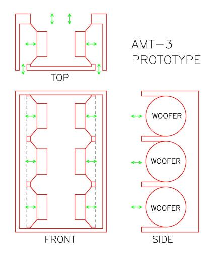
You will discern several things from the diagram, among them that I was not employed as a draftsman. What I hope you can make out is an arrangement where three woofers on each side fire into a flat surface and the pressure generated flows out the front through a vertical slot. The rear wave of the woofers is allowed to amble out rear of the enclosure. These were 8 inch woofers, which gives you an approximate sense of the scale.
