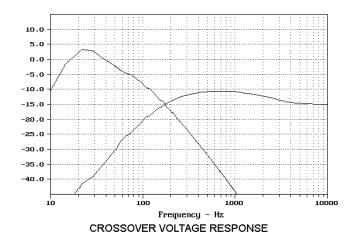
Notice that more gain is required for the bottom end, although if you're not crazy about bottom end you can probably get by with wiring the woofers for 5 ohms, which will give you most of the difference if you want to run passive crossovers. Here's the acoustic response:
