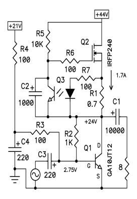
You can see a constant current source provided by Q2, R1, R5, R6, R7, C2 and an opto-isolator Q3 used as a current regulator. This circuit provides a relatively constant amount of DC current to bias Q1, the transistor of interest. Current through R1 develops about 1.1 volts across the LED portion of the opto-isolater which emits light that turns on the photo sensitive transistor of Q3 and this forms a feedback loop around Q2 which regulates the current.
