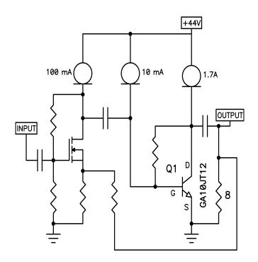
This should not be considered the best possible circuit, but is intended to illustrate an approach where a current source input and feedback to the GA10JT12 might be simply achieved. Alternatively, you can control the bias and feedback with an op-amp circuit.
